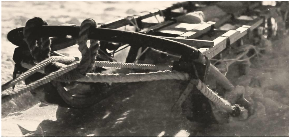
Detail of Nansen sledge showing arrangement of towing pennant and rope brake
