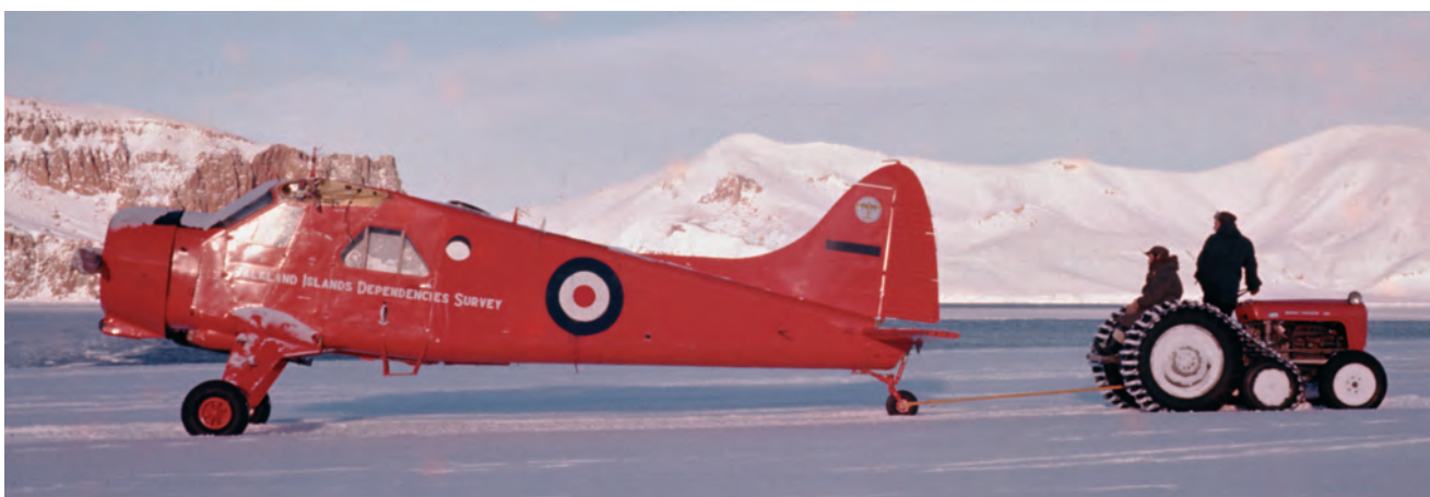
Below: In 8.60 VP-FAJ was repaired and converted to a wheel/ski land-plane at Deception Island following an unfortunate wing-bumping accident on 12.3.60. Seen being hauled from the repair hangar at Deception, it has the recently-applied full FIDS titling on the fuselage and taped-over registration on the fin. (M H Tween/BAS/Crown©)
