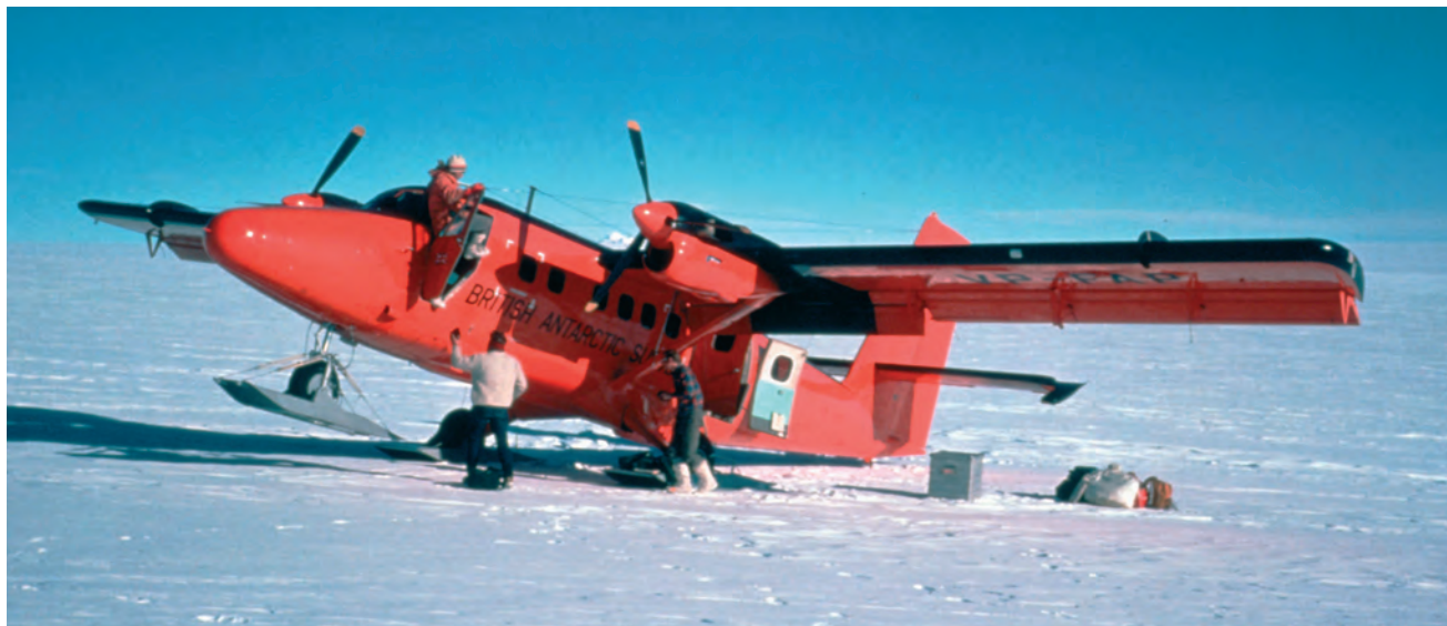
Above: Twin Otter Series 300 VP-FAP in an interesting 'nose-up' attitude clearly displaying its underwing registration and the nosewheel ski fitting. (P Prattis/NERC©)
