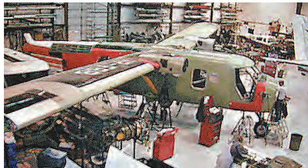
Above: VP-FBB under reconstruction in the hangar at Calgary; the red coloured panels are reutilised bits of original airframe, the two-shades-of-green sections are a combination of refurbished and new portions. (BAS / NERC © )
