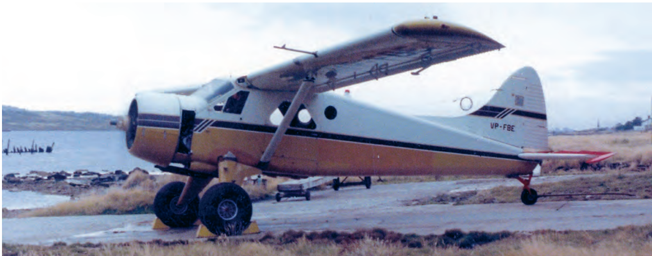
Above: Fitted with Tundra tyres, VP-FBE operated very successfully as a landplane for nearly a year before it was withdrawn from service in 1.85 and sold - thus ending an era which stretched back to 1953 when the first FIGAS Beaver entered service. (V Steen)
