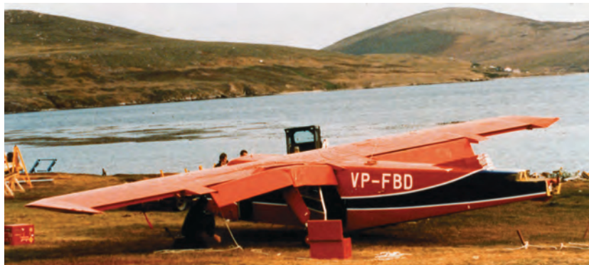
Above and Below: Following its landing accident at New Island (West Falkland) on 2.1.92, FIGAS BN-2B-26 Islander VP-FBD was gradually dismantled and shipped back to Stanley Airport for a protracted repair and return to service. (Author's Archive)
