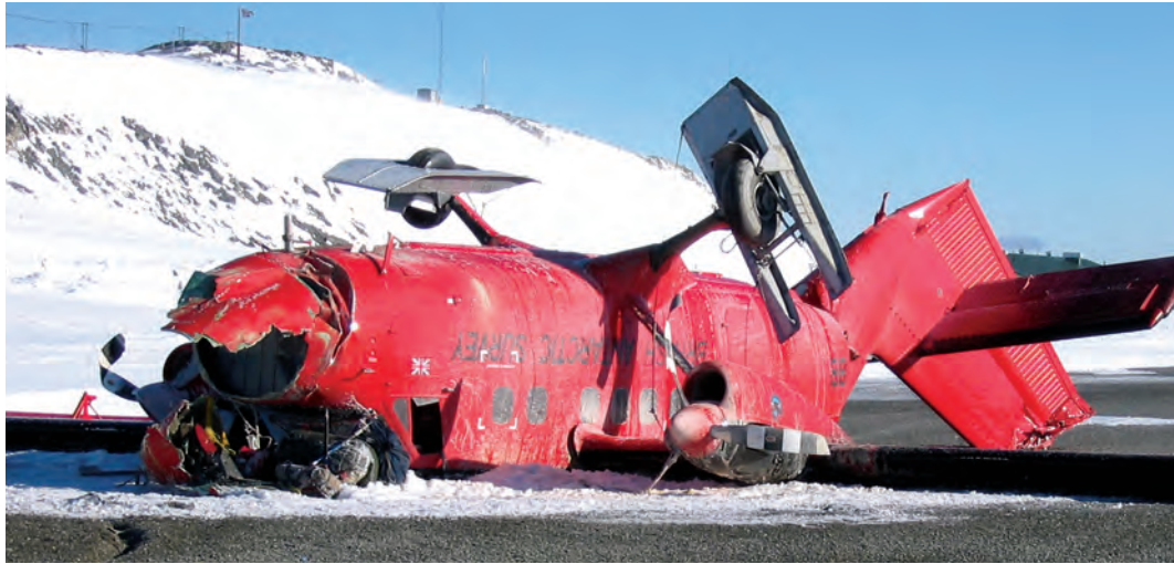
Left: "Its a write-off!"...is a perfectly understandable conclusion when viewing the upside-down and mangled airframe of BAS DHC-6 Twin Otter VP-FBB which had been flipped over by a sudden 40kt crosswind whilst landing at Rothera on 7.11.03. Remarkably it was deemed repairable and shipped to Rocky Mountain Aircraft at Calgary (Springbank) airfield, Canada, for a complete rebuild. (BAS / NERC ©)
