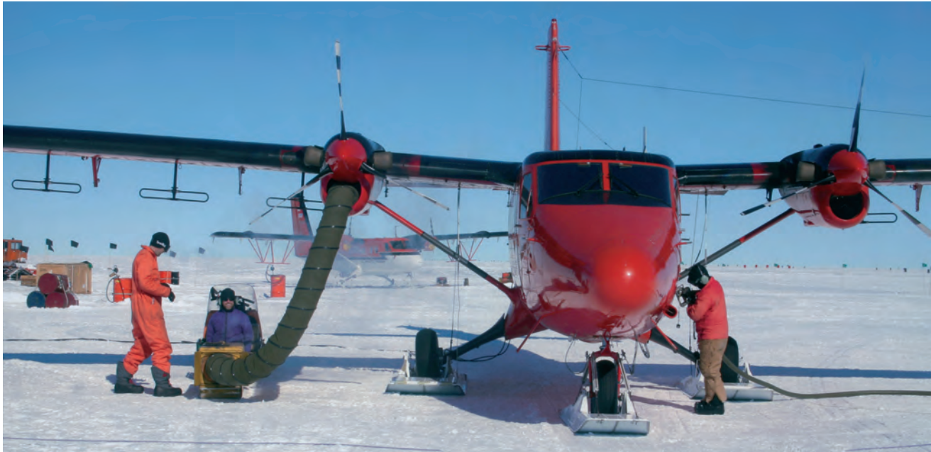
Above: Engine start - the Antarctic way! Because of the extreme cold, hot air is drawn into the engine prior to start-up. The aircraft involved is BAS Twin Otter VP-FBL with a Canadian example belonging to Kenn Borek Air Ltd in the background. (David Leatherdale/BAS/NERC ©)
