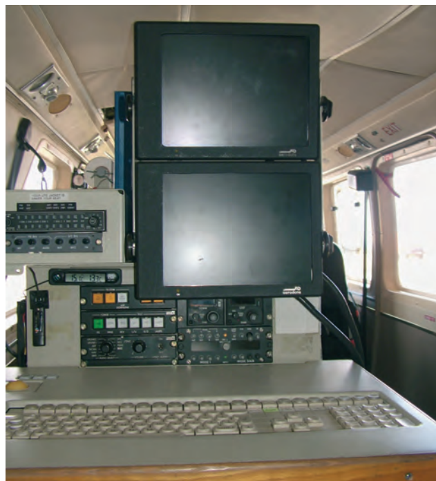
Above: For Calibration duties, a Flight Inspector's station is installed inside the Islander's cabin which necessitates removal of some standard Patrol fittings. (Morgan Goss)
