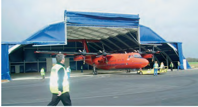
Above: On its return to Kidlington on 14.4.06 a welcome sight for BAS DHC-7 VP-FBQ was an Ably Shelters Ltd relocatable hangar. This allowed under cover maintenance and storage there for the first time. Although primarily intended for the Dash 7, it can also be used for Twin Otter servicing. (BAS/NERC ©)
