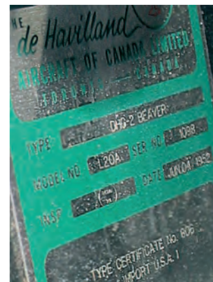
Above: Data plate of C-FHVT showing Model L20A and Ser.No. 1098. (Neil Aird)
